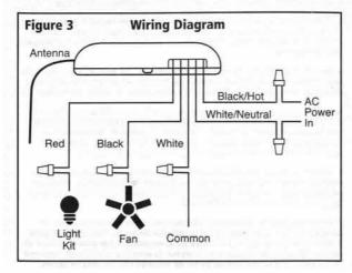
Low Profile Style II (Fig. 2-D): Secure receiver to the ceiling mounting bracket with UL listed cable ties (not included). Connect wiring as shown in Figure 3. Extend antenna above the ceiling mounting bracket (approximately 3-6).
